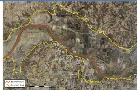
The BSNP structures highlighted in red, constrain the river channel.
