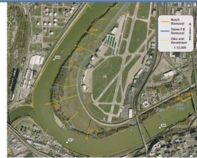
Dike modifications between the years 2004 and 2013 near the Downtown Kansas City airport. These modifications were needed because of ongoing bed degradation.
